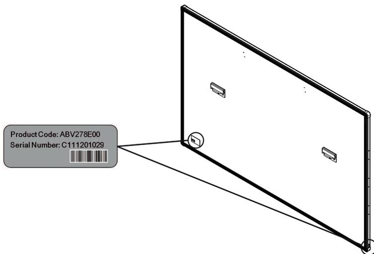
The label can be found on the rear of the board, at the lower left hand corner of the ActivBoard and lower side edge.
