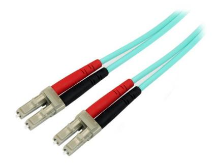
This fiber optic cable lets you connect 40GBase-SR4, 100GBase-SR10, SFP+ and QSFP+ transceivers in 40 and 100 Gigabit networks. The OM4 cable supports Vertical Cavity Surface Emitting Laser (VCSEL) and LED light sources and is backward compatible with your existing 50/125 equipment.
