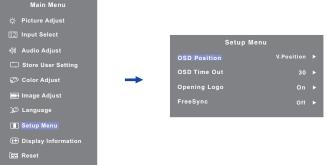
An adjustment page appears after you press the ENTER Button. Then, use the  $\P$  /  $\blacktriangleright$  Buttons to change the OSD vertical position settings. The OSD vertical position of the overall display should be changing accordingly while you are doing this.
