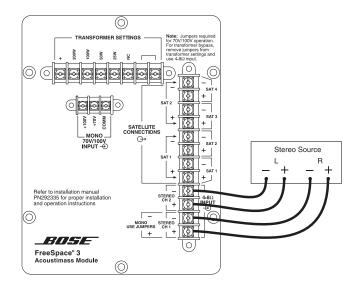
**Please note:** In setting up this operation, the following situation may occur: During system testing, while the source drives one channel only (shown right), a reduced output from the other channel is audible.
