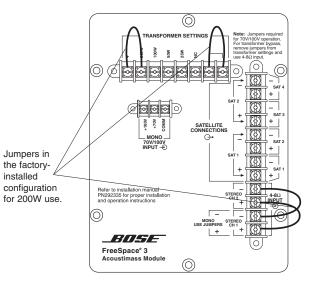
The transformer tap setting from the factory is for 200W use. To set it for lower wattage, remove the end of the '+' jumper wire connected to 200W and reattach it to the appropriate tap (100W, 50W or 25W).
