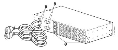
**Power cords:** The two cords connect the ATS to two separate power sources (A, B). The switch draws power from the preferred source and automatically switches to the secondary source when necessary. The two (2) 2.44-m (8-ft) power cords have IEC-309 32 A plugs.
