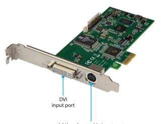
A/V breakout cable input port (For component, s-video, and composite video input + RCA audio input)
