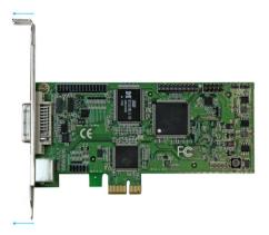
4. Line up your desired bracket so that the DVI input port, and the A/V breakout cable input port align with the port holes. Also ensure the screw hole is aligned with the underside of the capture card.
