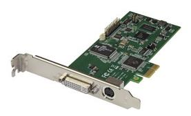
This PCIe video capture card lets you record 1080p HD video and 2-channel stereo audio (HDMI/RCA) to your computer system. With multiple video inputs, including HDMI, DVI, VGA and component, this all-in-one capture card can record original content from virtually any device.
