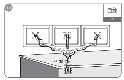
Insert cables into cable covers. Leave enough slack of cables at arm joints for fully adjustment. Use cable clamp to limit cables close to steel pipe.
