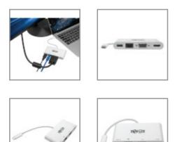
USB-C adapter connects an HDMI or VGA monitor, USB peripheral and wired Gigabit Ethernet network to a USB-C or Thunderbolt 3 device.
