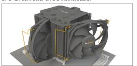
When dismantling the fans, push the notches of the fan clips (18) away from the fan.
