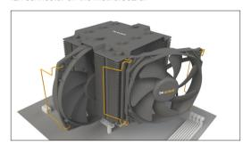
When dismantling the fans, push the notches of the fan clips (18) away from the fan.
