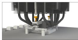
Fasten the 120mm fan (3) using fan clips (18) onto the front side of the cooler. Slide the 135mm fan (2) between the two heatsinks and also fasten this with fan clips (18). Connect both fans using the Y cable (20). Connect this to the CPU fan connector on the motherboard.
