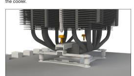
Fasten the 120mm fan (3) using fan clips (18) onto the front side of the cooler. Slide the 135mm fan (2) between the two heatsinks and also fasten this with fan clips (18). Connect both fans using the the Y cable (20). Connect this to the CPU fan connector on the motherboard.
