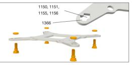
For fixing the backplate screws onto the Intel backplate use the O-rings (14). Once assembly of the Intel backplate for the respective Intel socket is complete, position it under the
