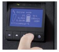
9SX LCD tilts 45° for ease-of-viewing
