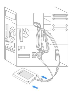
**Step 4-** The Solid State Drive can be securely mounted with the screws provided.
