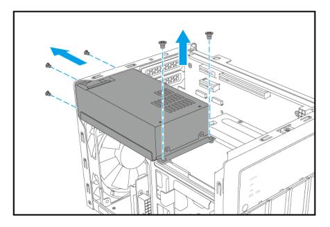
**c.** Remove the unit from the chassis.
