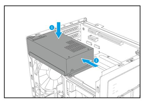
**b.** Attach the screws that secure the unit to the chassis.
