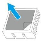
**c.** Install the heatsink on the controller.
