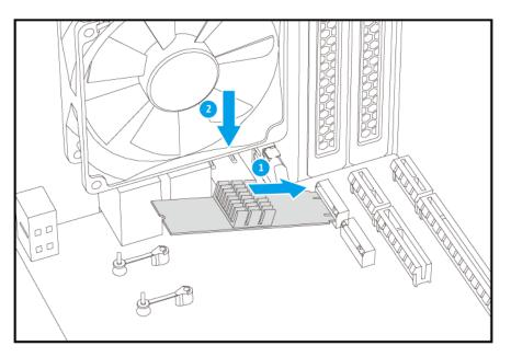
**c.** Insert the pushpin to secure the drive.
