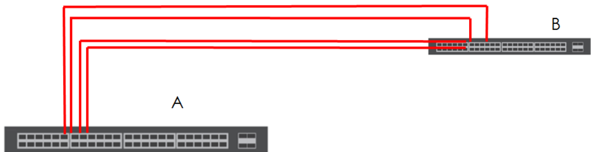
Figure 127 Trunking Example - Physical Connections
