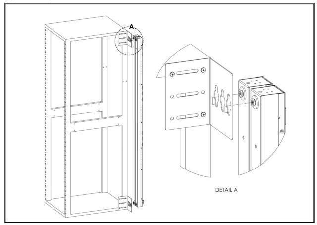
Figure 2.7 Offset/Side Mount Brackets
