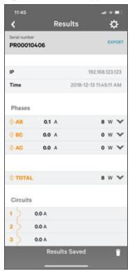
NOTE: The unit serial number is displayed in the title bar of the Readings page. This serial number matches the serial number located on the surface of the rPDU.
