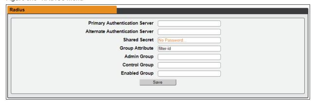
Primary Authentication Server: Enter the IP address of the primary authentication/authorization/accounting server. The Primary Authentication Server can be an IPv4 address, an IPv6 address in square brackets, or a host name. The Primary Authentication Server is used for authentication, authorization and accounting, and is required.
