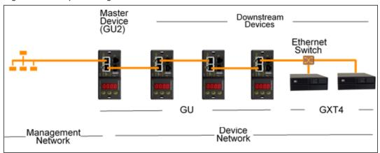
The IMD-3E is the default intelligence card for Vertiv Geist GU2 rPDUs, which include switched (model numbers beginning with MNR), outlet monitored (model numbers beginning with MNR), and switched plus outlet monitored (model numbers beginning with MNU) products. To serve as the master rPDU, rPDUs with a legacy intelligence card must first upgrade to the IMD-3E
