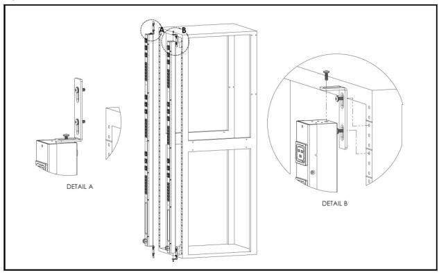
Figure 2.3 Vertical Extension Brackets
