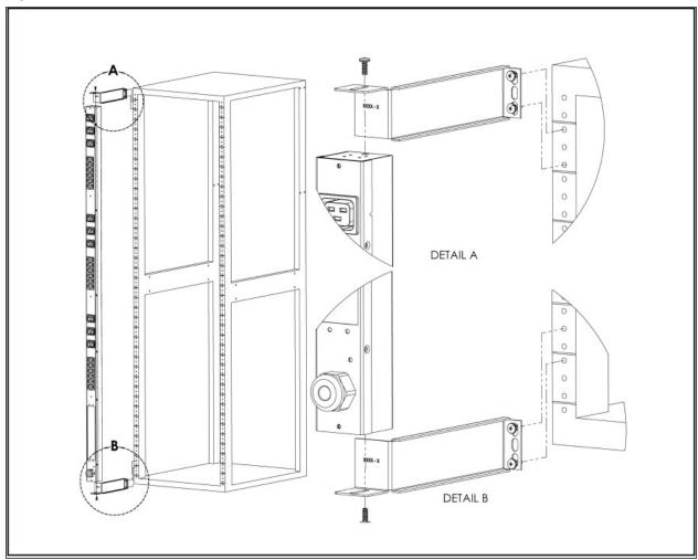
Figure 2.9 Flush Mount Bracket
