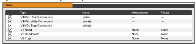
The Users section allows you to configure the various Read, Write, and Trap communities for SNMP services. You can also configure the authentication types and encryption methods used for the SNMP v3 if desired. Click the modify icon to change settings.
