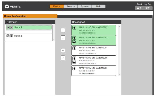
The Group Configuration page lists the automatically discovered devices under the "Unassigned" column showing:
