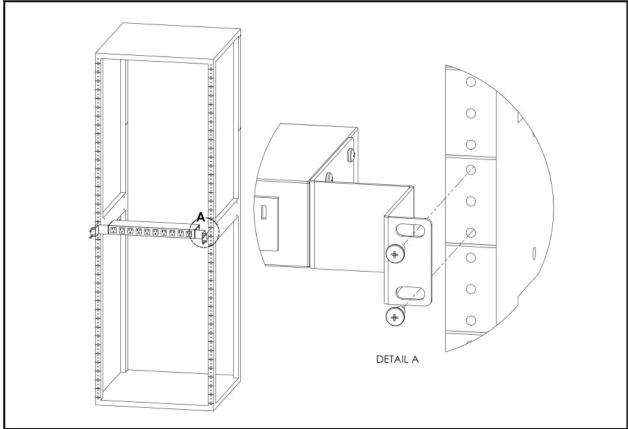
Figure 2.13 19" Horizontal/Panel Mount Brackets
