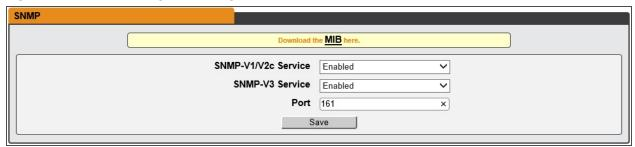
The SNMP-V1/V2c and SNMP-V3 Service can be enabled or disabled independently as desired. The service listens for data-read requests on port 161, which is the usual default for SNMP services; this can also be changed if desired.
