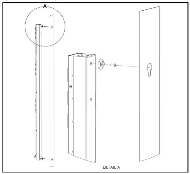
Figure 2.5 Toolless Full Length Brackets
