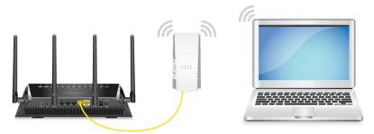
Figure 4. Extender in access point mode
