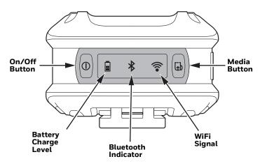
The front panel has an LED display and 2 buttons.
