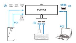
3. Enter to OSD menu. Go to KVM layer and select "Auto", "USB C" or "USB up" to switch the control of peripherals from one device to another. Simply repeat this step for switching the control system using one set of peripheral.
