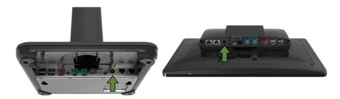
**3** Make additional connections from the bottom of the stand module or the Touchcomputer.
