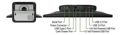
2 Make additional connections from the back of the Touchcomputer.
