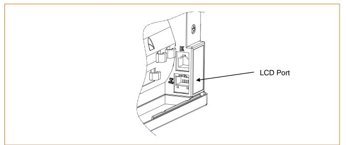
• Connect the BIXOLON Customer LCD Display BCD-3000 cable to the LCD connector located at the rear of the printer.
