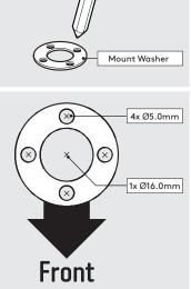
Using the Mount washer, **A1** mark the drill hole locations as shown.
