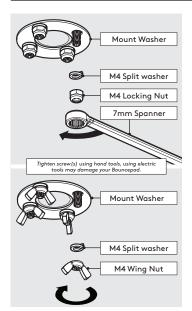
Secure the arm to the A4 surface. Locking Nuts offer higher security.
