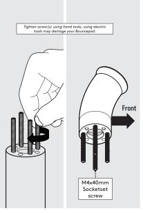
Locate and screw the Socket screws into the Desk as shown
