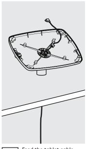
Feed the tablet cable through the Bouncepad Case & Flex.
