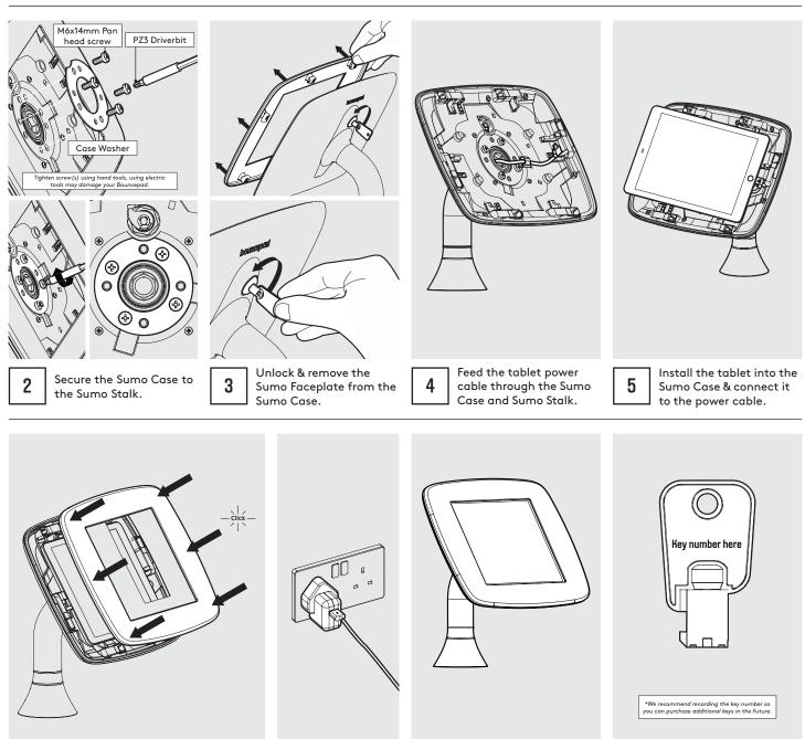
Locate the Sumo Faceplate onto the Sumo Case - pressing the Faceplate firmly down to ensure correct locking.
