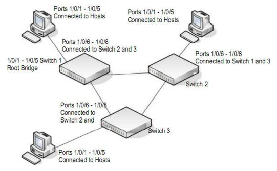
Figure 2. MSTP sample configuration
