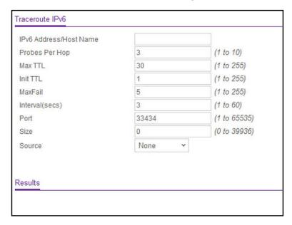
**6.** In the **IPv6 Address/Hostname** field, enter the IPv6 address or host name of the station to which you want the switch to discover a path.
