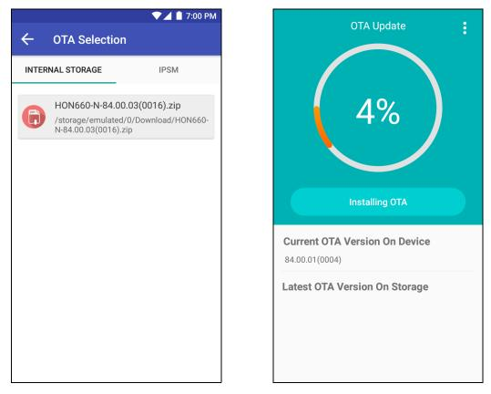
6. Once the installation is complete (100%), select **OK** when prompted to **Reboot** the computer. The computer reboots and finishes the update.
