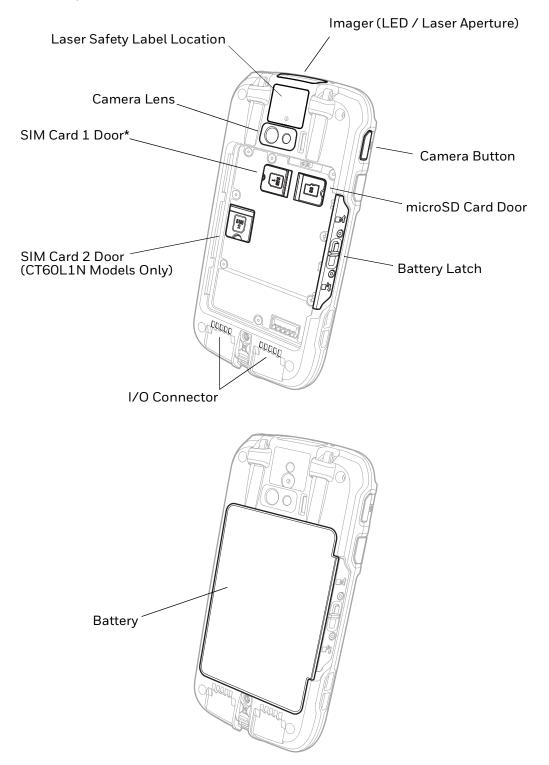
\* Phone feature is available only on CT60L1N models. For all models, when using a UICC card for NFC Secure Element NFC link encryption, install the card in SIM slot 1. SIM 2 feature is available only on CT60L1N models.
