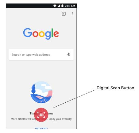
Tap and hold the button to activate the imager and scan a bar code.
