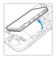
7. Lift up the edge of the SD card access door.
