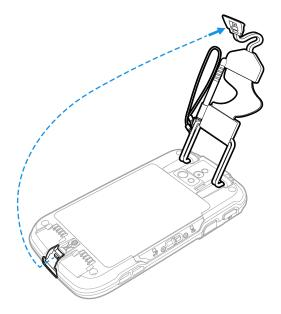
5. Press and hold down the small button on the battery latch, and then slide the latch toward the bottom of the computer to unlock the battery.
