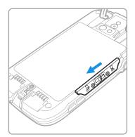
4. Lift up on the edge of the battery and remove it from the computer.
