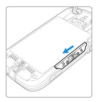
6. Lift up on the edge of the battery and remove it from the computer.
