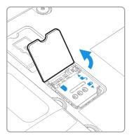
8. Press down gently and slide the card holder into the unlocked position. Lift the edge of the card holder up.
