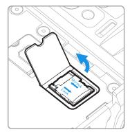
8. Press down gently and slide the card holder toward the open access door. Lift the edge of the holder up.
