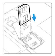
10. Close the holder with the card installed. Press down gently on the holder and slide it into the locked position.
