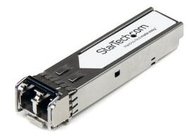
The JD092B-ST is a HPE JD092B compatible fiber transceiver module that has been designed, programmed and tested to work with HPE brand switches and routers. It delivers dependable 10 GbE connectivity over fiber cable, for 10GBASE-LRM compliant networks, with a maximum distance of up to 200 m (656 ft).
