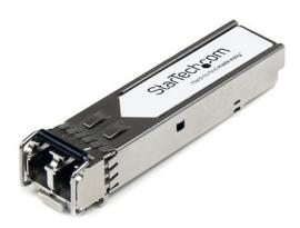
The AR-SFP-10G-SR-ST is an Arista Networks SFP-10G-SR compatible fiber transceiver module that has been designed, programmed and tested to work with Arista Networks brand switches and routers. It delivers dependable 10 GbE connectivity over fiber cable, for 10GBASE-SR compliant networks, with a maximum distance of up to 300 m (984 ft).
