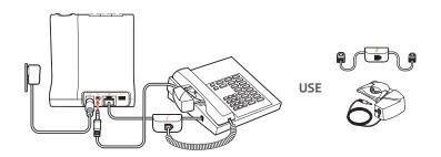
**IMPORTANT** *Cisco* phones use configuration **D** on the bottom of the base. Most other phones use default configuration **A**.
