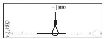
Pulling a Cable Lock Through the Laptop Lock's Loop
