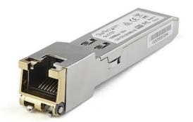
The SFP1GETST is a Juniper SFP-1GE-T compatible copper transceiver module that has been designed, programmed and tested to work with Juniper brand switches and routers. It delivers dependable 1 GbE connectivity over copper cable, for 10/100/1000BASE-TX compliant networks, with a maximum distance of up to 100 m (328 ft).
