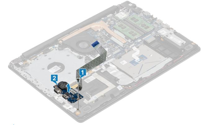
() NOTE: When the IO board cable is disconnected from the system board, an RTC error occurs. This error occurs whenever the RTC/coin-cell battery, IO board, or system board are removed.
