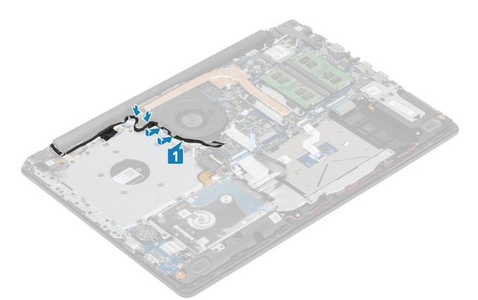
4. Connect the ODD cable, display cable and fan cable to the system board [3,2,1].
