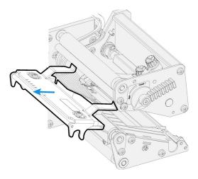
8. Disconnect the cables from the printhead. Note the snap-lock on the inner connector. Pull at the connectors, not at the cables.
