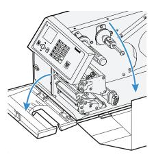
3. Turn the printhead lift lever counter-clockwise to raise the printhead.
