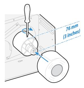
7. Fit a new roll of media onto the media supply hub and push the roll in as far as it will go.
