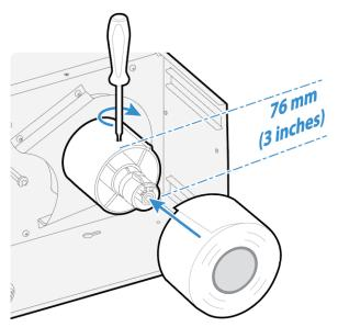
8. Fit a new roll of media onto the media supply hub and push the roll in as far as it will go.
