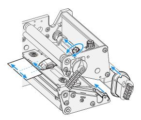
5. Move the pressure arm inward or outward until the arrow on the tip of the arm is centered with the media.
