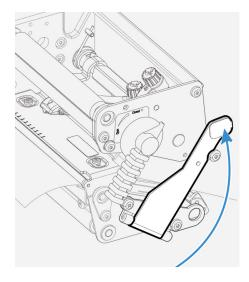
12. Adjust the position of the red edge guides so that the media is guided with a minimum of play.
