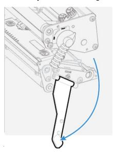
3. Turn the printhead lift lever counter-clockwise to raise the printhead.
