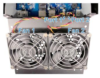
**Note:** Please insert the fan power cords to their corresponding ports. As illustrated above, attach fan 1 to port 1. This may influence the fan numbers displayed on the system when a fan malfunction occurs.
