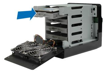
Note: Make sure the drive tray is completely inserted. Otherwise, the drive might not be able to function properly.
