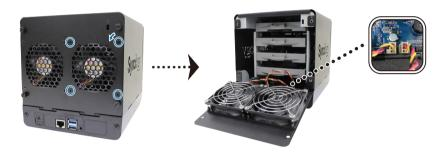
4 Remove the fan guard and replace the malfunctioning fan with a new one.
