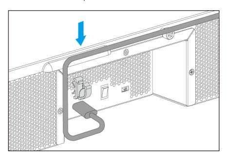
**3.** Close the clip to secure the cable.
