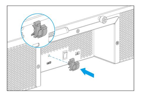
2. Insert the cable into the clip.
