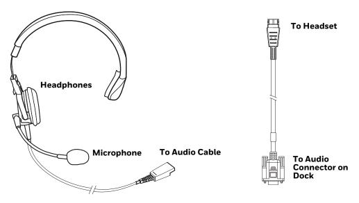
See Audio Connector for connector pinouts.
