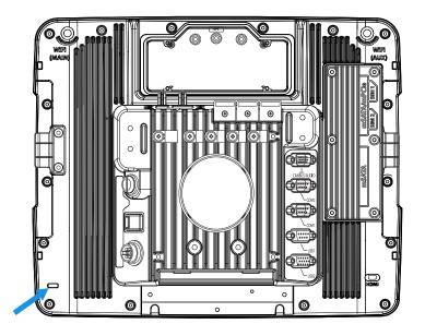
The VM3A can be secured with a standard laptop security cable using the slot on the back.
