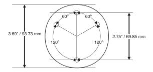
Attach the RAM ball base to the vehicle mounting surface using three or four 1/ 4 bolts (not included) or equivalent fasteners. If the mounting kit includes cone washers, use those as illustrated below.
