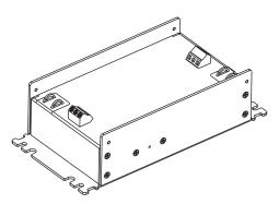
Shown with Lid Removed Input and output connector blocks under lid. One positive (VIN+), negative (VIN-), and ground
