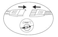
Adjust Headset/Microphone and Secure Cable
