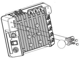
2. Attach the RAM ball to the back of the scanner holder.
