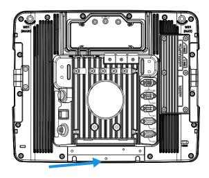
It may be desirable to secure the VM3A in the dock so it cannot be removed from the dock. The quick release handle on the computer is notched to allow a user supplied small padlock to be placed through a hole in the bracket on the back of the computer in the location shown below. Once the padlock is installed, the release handle cannot be moved so the VM3A cannot be removed from the dock. The padlock shackle must be smaller than 3/16" (4.76mm).
