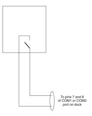
Pins 7 and 8 must be connected as shown in the illustration above. No other pins are to be connected.
