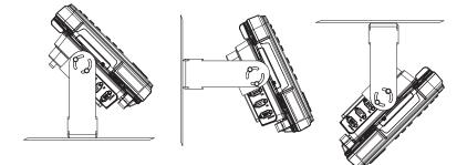
Step 4. Install U Bracket to Vehicle
