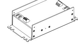
Shown with Lid Attached Lid is secured with screws on the side of lid.
