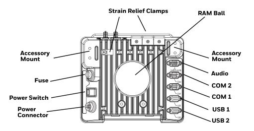
**Note:** For the VMX Enhanced Dock: COM1 is used for screen blanking (via the power cable connector) and is unavailable when the screen blanking box is attached. When a screen blanking box is attached, any external serial device, such as a scanner, must be connected to the COM2 port on the dock. If a screen blanking box is not connected via the power cable, the COM1 port on the dock is available for a serial device.
