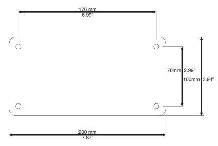
3. If not already attached, attach the RAM ball to the RAM ball plate using three M6 nuts and washers.
