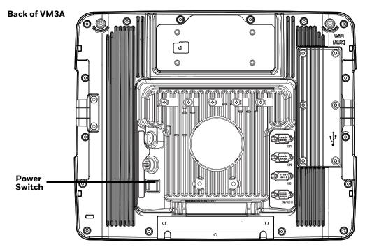
After external power has been connected and the computer has been mounted in the dock, press the side of the power switch with the raised bump to pass power from the dock to the computer.
