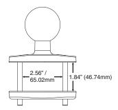
2. Position the upper clamp piece with ball on the beam. Place the bolts through the holes in the upper clamp piece. Position the lower clamp piece below the beam. Align the bolts with the holes in the lower clamp piece. Place the nylon locking nuts on the bolts and tighten the bolts.
