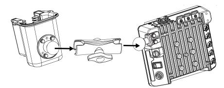
5. Tighten the knob on the RAM arm while adjusting to the desired angle.
