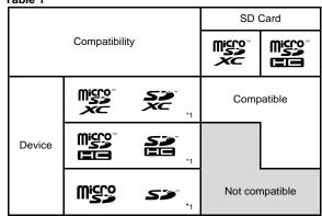
\*1 : Need an SD card adapter to use a microSDHC Card and a microSDXC Card.
