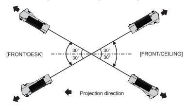
In the case of [AUTO], it will be detected as [FRONT/DESK] even when the projector tilts over  $\pm 30^{\circ}$  with the top side upward or over  $\pm 30^{\circ}$  with the top side downward. To use the projector that tilts over  $\pm 30^{\circ}$  with the top side downward, set the [PROJECTOR SETUP] menu  $\rightarrow$  [PROJECTION METHOD] to [FRONT/CEILING] or [REAR/CEILING] instead of [AUTO].
