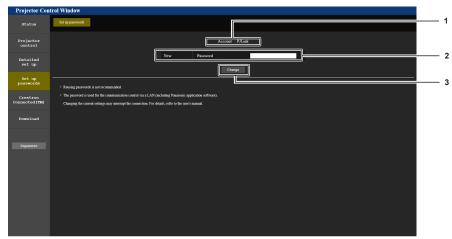
1 [Account: PJLink] Displays the account to change.  [New] [Password]: Enter the desired new password. (Up to 32 characters in single byte)
