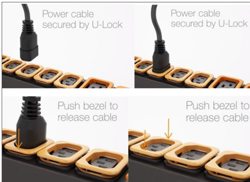
Figure 2.15 U-Lock Cord Retention Operation
