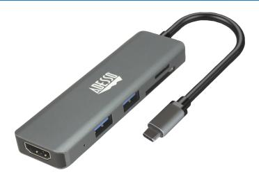
Expand your laptop's connection port with this USB Type-C multiport docking station. It has an HDMI port for transmitting 4K content to your external monitor and can also charge other devices. This USB Type-C multi-port docking station has 2 USB 3.0 superspeed ports and SD and TF card reader slots.
