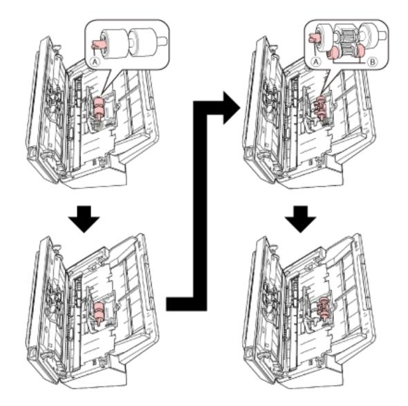
a Check the direction of the notch  $(\triangle)$  on the pick roller and of the small roller (B), and insert it in the hole.
