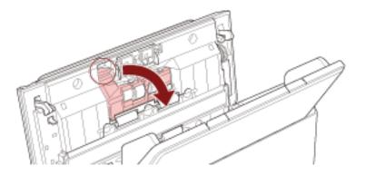
**b** Pull out the left side of the brake roller shaft, and then pull out the right side of the shaft from the hole.
