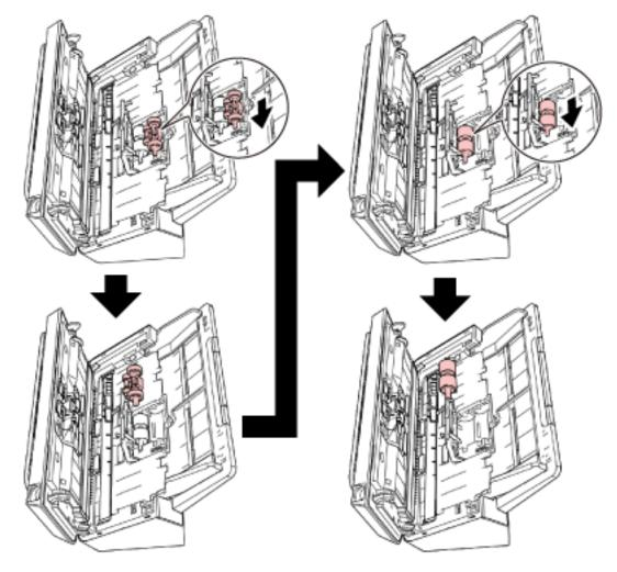
8 Attach a new pick roller from the bottom.
