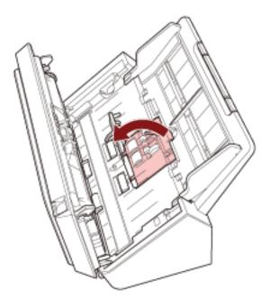
**b** Slide the pick roller and remove it from the top.
