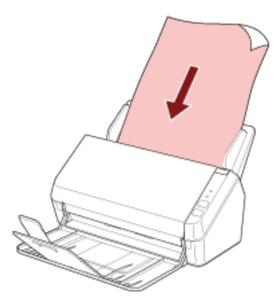
6 Adjust the side guides to the width of the Cleaning Paper.
