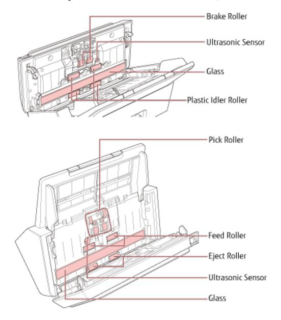
3 Clean the following locations with a cloth moistened with Cleaner F1, or a sheet of Cleaning Wipe.
