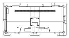
⑤ Attach the Stand to the monitor(VESA holes) and secure it in using the provided screws and screwdriver.
