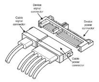
Each cable is keyed to ensure correct orientation. IronWolf drives support latching SATA connectors.
