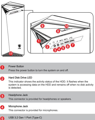
USB 3.2 Gen 1, the SuperSpeed USB, delivers up to 5Gbps high-speed data transfer for various devices, such as storage devices, hard drives, video cameras, etc. The slim and sleek USB Type-C connector features reversible plug orientation.
