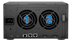
3 Remove the four screws that secure the fan panel.
