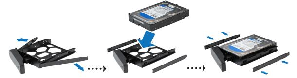
• For 2.5" drives: Remove the fastening panels from the sides of the drive tray and store them in a safe place. Place the drive in the area of the drive tray indicated by a blue rectangle below. Turn the tray upside down and tighten the screws to secure the drive in place.
