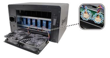
c Remove the screws that secure the fan from the fan case.
