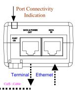
Figure 1: Connecting the PD-3501G
