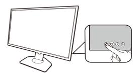
Turn on the computer too. If you have multiple video sources, press the Rotation key 2 and the 5-way controller to select an input source.
