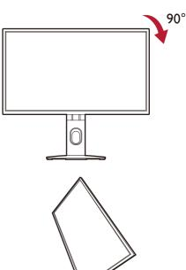
To avoid the edge of the LCD display hitting the monitor base surface while it is being rotated, do tilt and extend the monitor to the highest position before you start to rotate the display. You should also make sure there are no obstacles around the monitor and there is enough room for cables.
