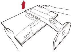
To move the monitor, you must hold the handle and the bottom of the stand base at the same time as illustrated. You can protect the monitor using the supplied dust cover.
