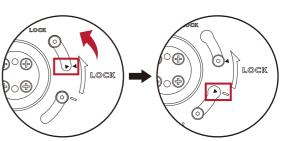
Raise the thumbscrew lids and tighten the thumbscrews as illustrated. Then push the lids back.
