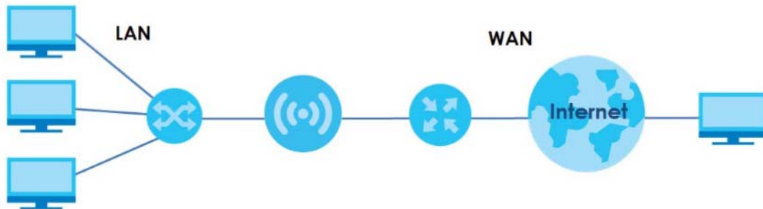
Figure 3 Internet Access Application: Ethernet WAN
