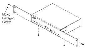
3. Use 4 self-supplied screw to secure the mounting brackets onto the rack.
