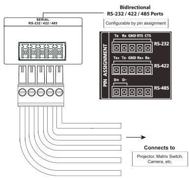
Connect to devices, configurable by pin assignments, for controlling and receiving status messages from them.
