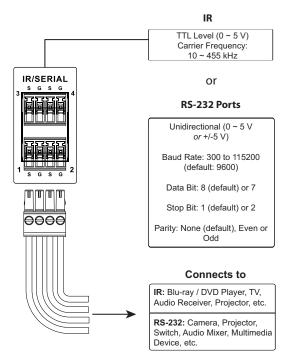
By default, the unidirectional IR / serial channels are set to transmit IR signals.
