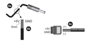
a) Cut the connector end of the power adapter cable.
