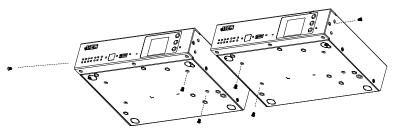
2. Use 4 of the screws from step 2 to secure the two VK1200 units together with the link bracket. Then install the left and right mounting brackets onto the sides of the units using 2 of the M3x5 and M3x6 screws included.
