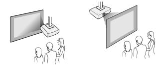
If you project from the ceiling or from the rear, select the correct **Projection** setting and, if necessary, adjust the **OSD Rotation** setting.
