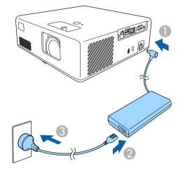
The projector enters standby mode. This indicates that the projector is receiving power, but is not yet turned on.
