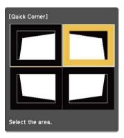
To reset the Quick Corner corrections, hold down for about two seconds while the area selection screen is displayed, and then select **Yes**.
